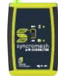
AIR CONNECTOR USED TO CONFIGURE THE LIGHTS WITH THE SYNCROMESH GATEWAY
